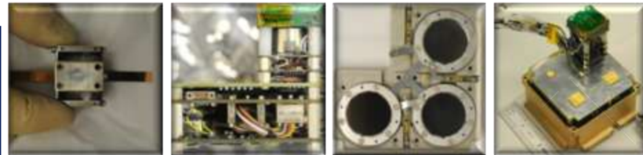
Flight Hardware for the SWATS instrument, from left to right: spectrometer body, flight electronics, focal plane array, anodes and HV power supply
