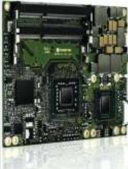
Skinless compute node for RECS (2 or 4 cores, max. 16 GB RAM)
