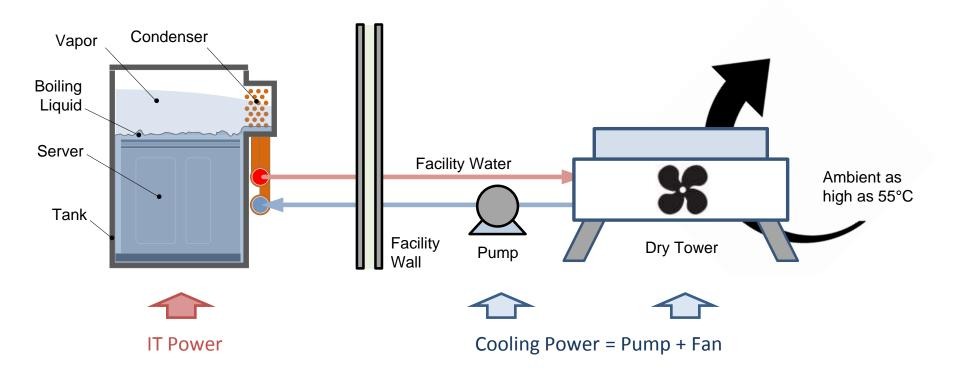
OBI does not require: chillers, cooling towers, water use, raised floors, computer room air conditioners or earplugs!
