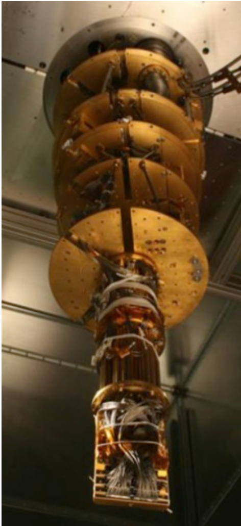
Cryogenics (10 kg of metal at 15 milliKelvin)
