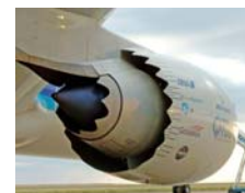
Advanced chevron nozzle installed on B777 for NASA/Boeing QTD-2 flight test
