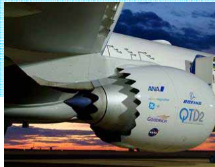
2005 QTD 2 Quiet Technology Demonstrator Boeing General Electric Goodrich NASA All Nippon Airlines
